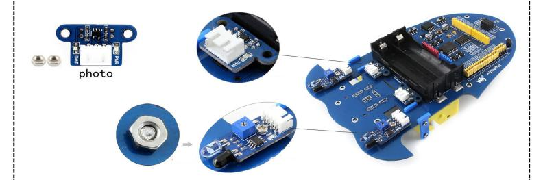
Connect a XH2.54 4cm 4Pin cable to the Infrared sensor, and tie a XH2.54 4cm 3Pin cable to the Photo sensor.
