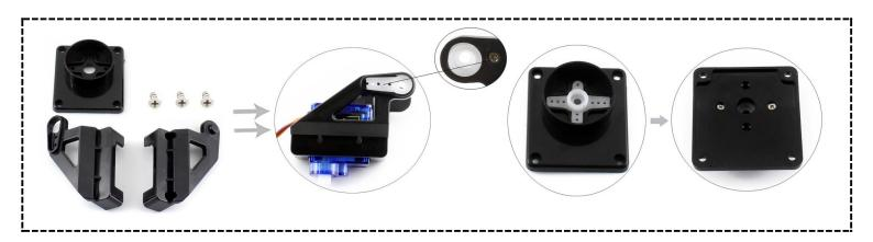
Insert the steering gear describe above to cross-shape rocket arm (b.) in the stand (d.) and fix the installation with a screw (1.). Fix another steering gear into the stand (e.), and fix it with two screws (7.). Install the stand (e.) and steering gear to the stands (f.) and (g.), and fix them with the screw (1.).
