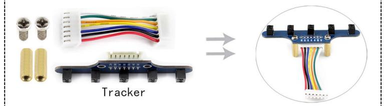
And then, connect the XH2.54 4cm 7Pin cable described above to the AlphaBot baseboard, and fix the Tracker senor to the AlphaBot baseboard with (B).
