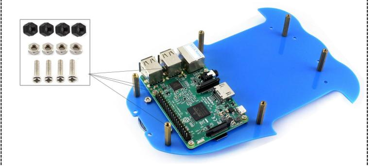
Install the camera pad&tilt unit to the front end of the AlphaBot baseboard, and fix it with (6.) and (4.). Pass the camera cable through the flat cable hole and connect it to the Raspberry Pi board. Fix the Acrylic baseboard to the AlphaBot baseboard with (B).
