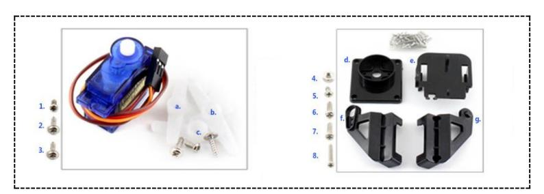
⑤ Place the steering gear in the middle of the stands (f.) and (g.) and fix it with the screw (7.). Please make sure the rotor on the steering gear is installed in a correct direction.
