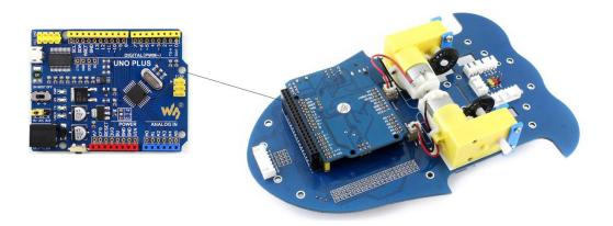
Fix the completed ultrasonic unit to the AlphaBot baseboard with (B), and connect a XH2.54 20cm 4Pin cable to the ultrasonic Pinboard. (Connect the steering gear to the S1 interface with the cables, in which the black line is to the brown port, the red line to the red port, and the yellow line to the yellow port.)
