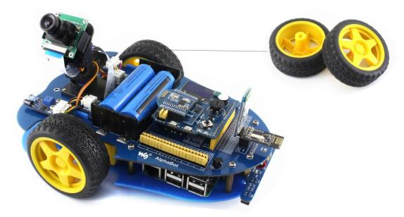
In additional, Arduino and raspberry Pi can work together at a same time in a same car via serial communication.
