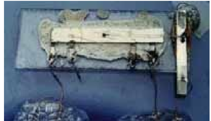
The first integrated circuit, TI
