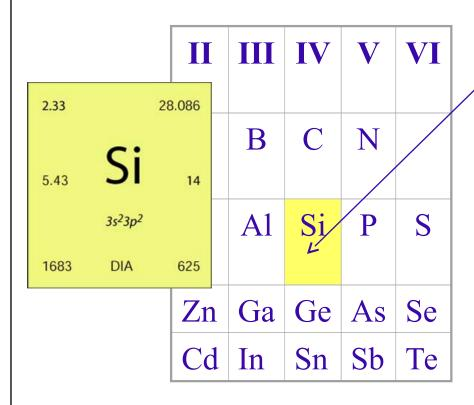
Silicon (Si) – the dominating material in IC manufacturing
