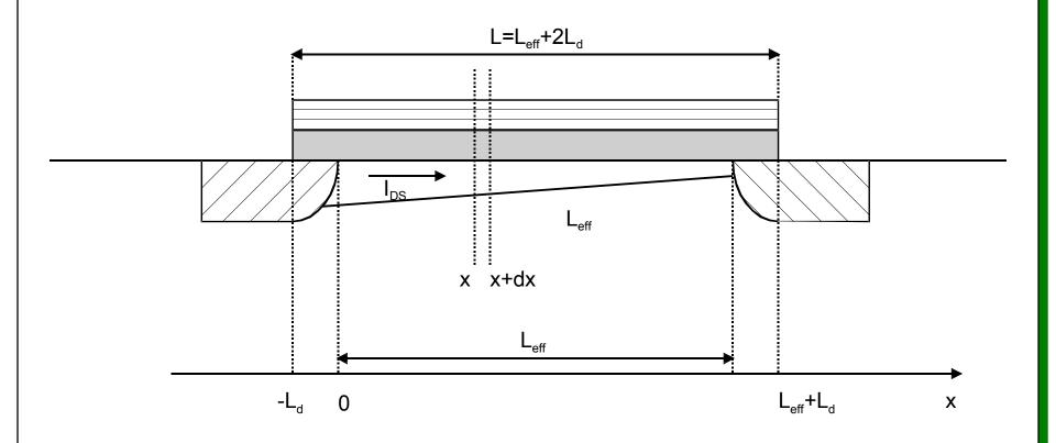
$$I_{DS} = \mu \frac{W_{eff}}{L_{eff}} C_{ox} \int_{0}^{U_{DS}} (U_{GS} - V_{T0} - V(x)) dV$$
