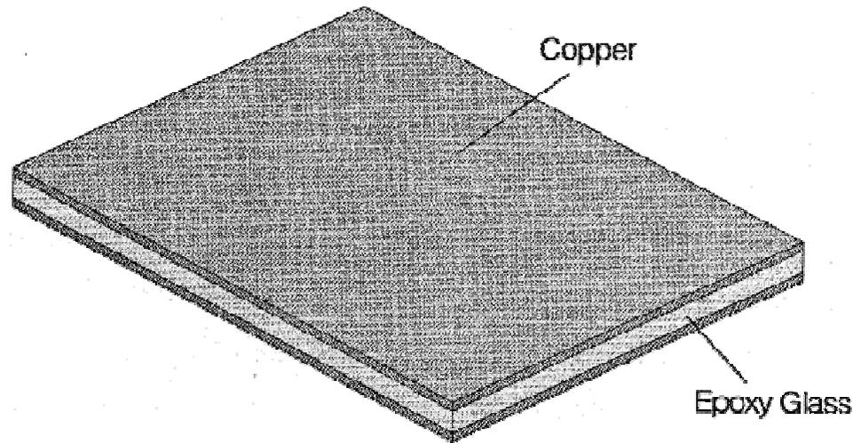
(1) *Copper-clad epoxy glass*
