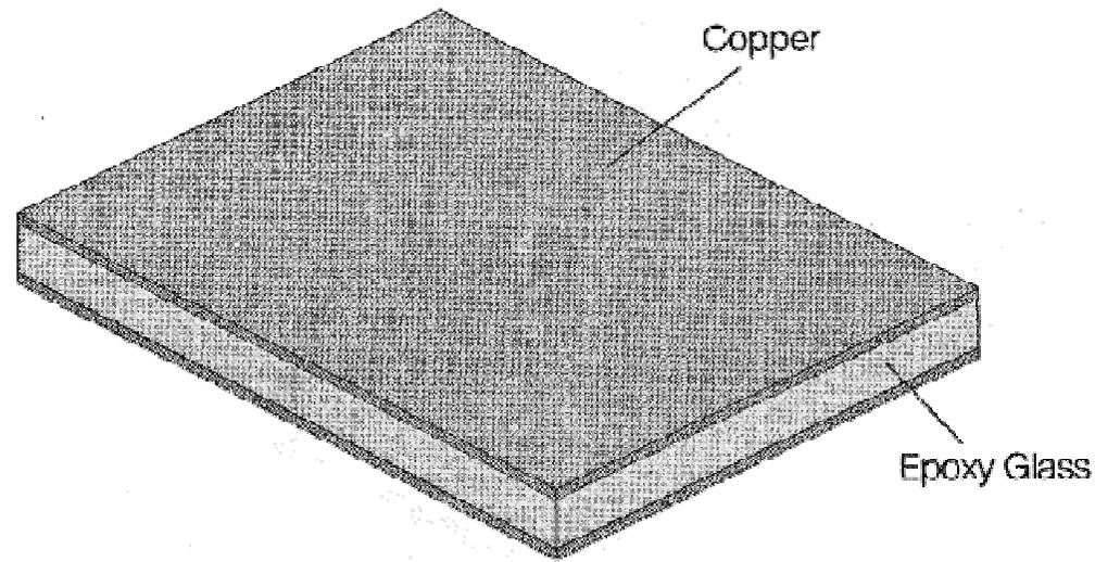
*(1) Copper-clad epoxy glass*
