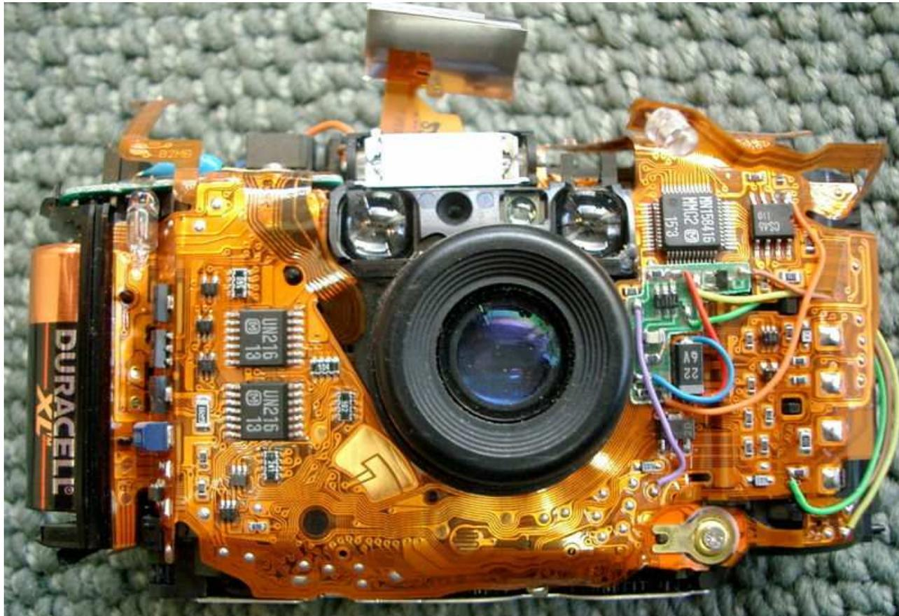
Olympus Stylus camera with skins removed, showing flex circuit assembly
