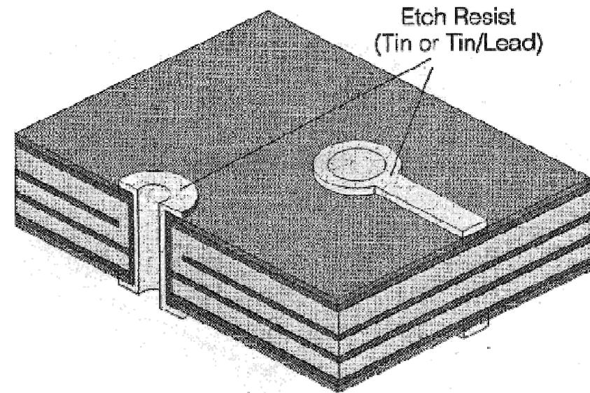
(10) *Electroplate etch resist*
