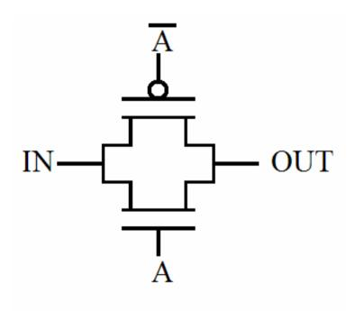
$R_{on} = 100\Omega$  and  $R_{off} > 5~M\Omega$  (high impedance H)
