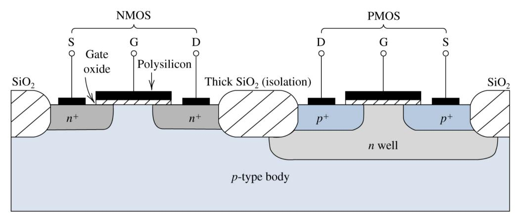
Note that the PMOS transistor is formed in a separate *n*-type region, known as an *n* well. Another arrangement is also possible in which an *n*-type body is used and the *n* device is formed in a *p* well.
