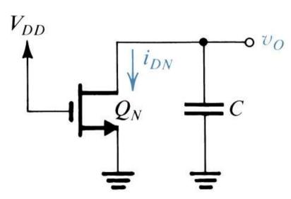
equivalent circuit during the capacitor discharge.
