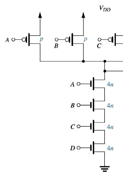
Proper transistor sizing for a four-input NAND gate.
