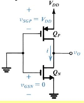
circuit with v1 = 0V (logic-0 level, or  $V_{OL}$ );
