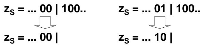
FP working registers must be longer then the nominal size to provide higher accuracy as long as possible, before rounding.
